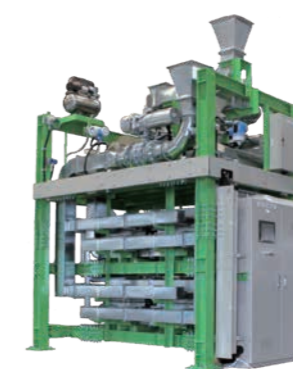
New ventilation system using a gas-permeable membrane (Demonstration machine)
