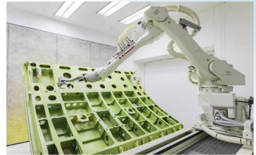
Cutting-edge technologies and solutions coupled with the suriawase * approach enable Kawasaki to achieve sophisticated product manufacturing. (The photo shows Kawasaki robots producing cargo doors for the Boeing 777X at Kawasaki Motors Manufacturing Corp., U.S.A.)
