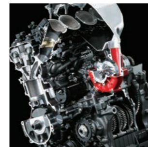
Supercharged engine for large motorcycles (Ninja H2R)
