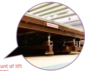
How the tatami unit is elevated: The blower injects air into the balloon-like bag (air mat), and the bag swells and elevates the unit about 40 mm. The unit has myriads of holes at the bottom, and as the air escapes through these holes, a layer of air beneath the bag is also created, reducing the friction between the tatami unit and the floor to one thousandth.
