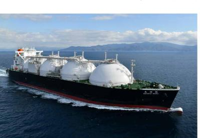
via the Freeport LNG Project in the U.S. The vessel features standard LNG carrier hull dimensions in order to enable docking at major LNG terminals around the world while offering larger cargo tanks for increased transport capacity, thus cutting LNG transport costs and facilitating more flexible LNG trade operations by shipowners.
