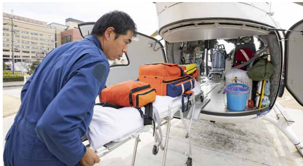
Rear clamshell doors secure enough space for loading/unloading the patient. The height of the cabin floor is configured to make it easy to stretch out the stretcher’s legs.
