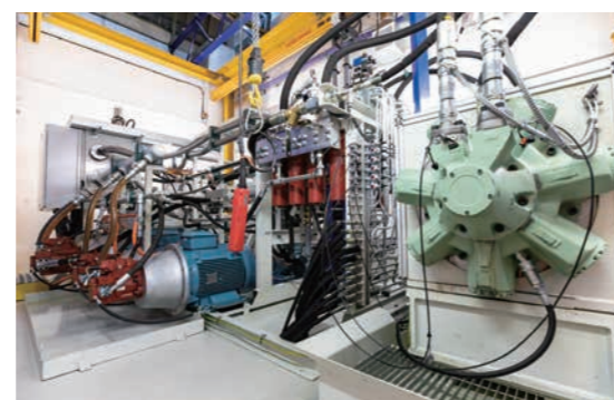
(Photo above) A hydraulic pump being assembled at the Plymouth plant. Most key components are imported from Japan or sourced within the EU, but KPM (UK) also manufactures some of the parts. (Upper right) Casing for hydraulic pump awaiting assembly at the Plymouth plant after being imported from Japan. (Lower right) In the testing room for new products, a Staffa motor on the right and a hydraulic pump on the left undergo operational tests.
