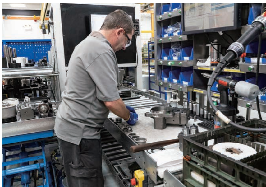
(Photo above) A hydraulic pump being assembled at the Plymouth plant. Most key components are imported from Japan or sourced within the EU, but KPM (UK) also manufactures some of the parts. (Upper right) Casing for hydraulic pump awaiting assembly at the Plymouth plant after being imported from Japan. (Lower right) In the testing room for new products, a Staffa motor on the right and a hydraulic pump on the left undergo operational tests.
