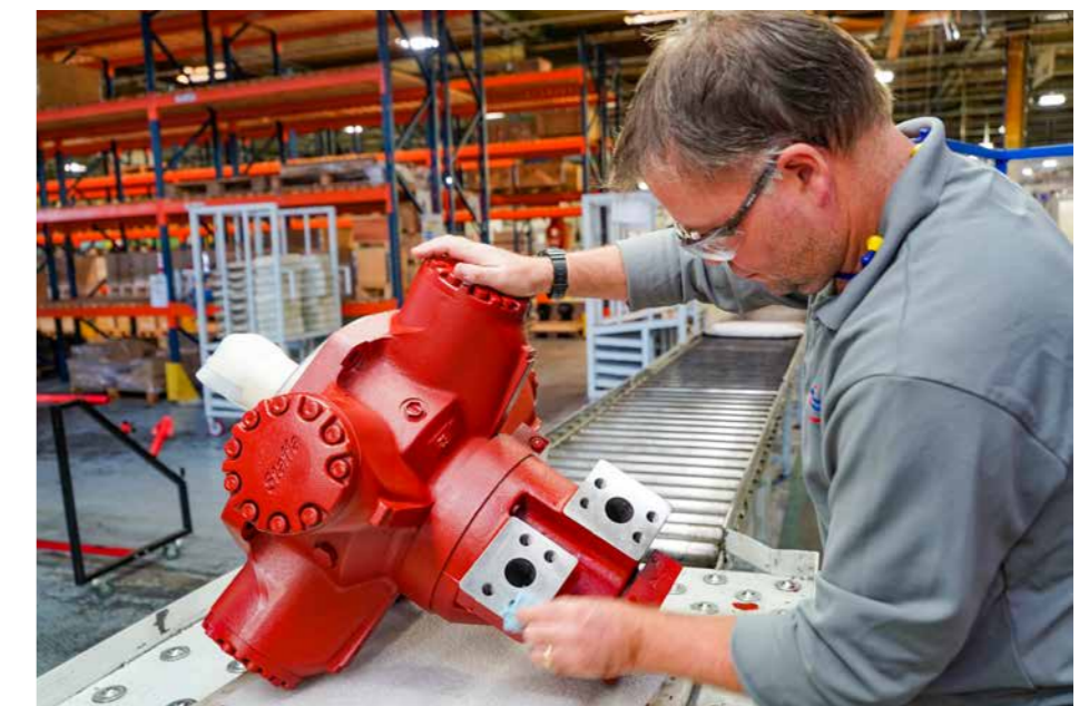
Staffa motor undergoing a finishing process.
