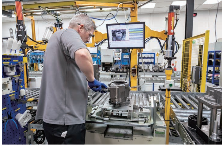
Instructions for assembly are displayed on the LCD monitor, making it a paperless procedure. This method was first utilized for hydraulic pumps, but it is now applied to Staffa motors.
