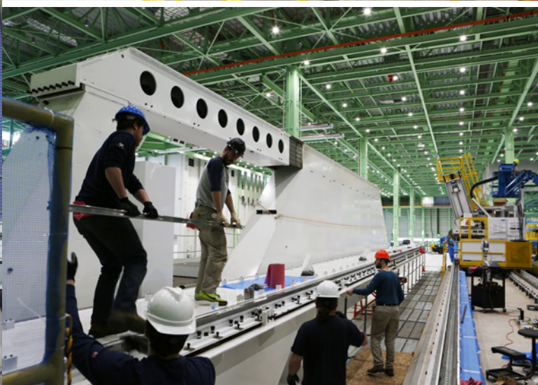
East Plant gets ready for full operation (bottom right). Adjustment of the AFP machine, which forms composite layups (top left), and installation of the panel riveter (bottom left) are also underway. Picture at top right shows the combustion system and other parts of the autoclave extending outside the facility.
